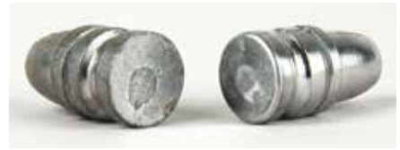
One defect in revolver bullets (above) Duke will not accept is a rounded base such as the sample at right. Bullet at left has a perfect base. Duke's favorite .44-40 bullet (below) is RCBS #44-200-FN. Note top-left bullet has rounded bands. Duke considers it still fine for revolver shooting.
