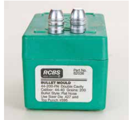
One defect in revolver bullets (above) Duke will not accept is a rounded base such as the sample at right. Bullet at left has a perfect base. Duke's favorite .44-40 bullet (below) is RCBS #44-200-FN. Note top-left bullet has rounded bands. Duke considers it still fine for revolver shooting.
