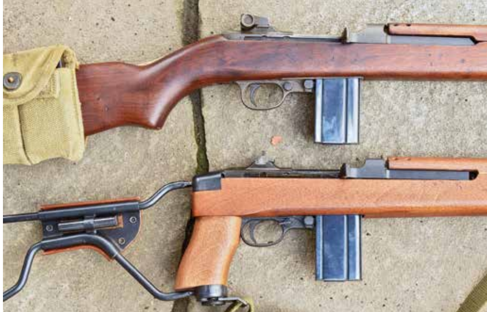
Carbines were continuously updated. The upper carbine has an early push-button safety and improved milled rear sight while the lower has a late war rotating safety and an early two-leaf, flip rear sight.
