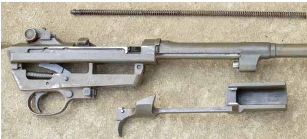
The entire barrel, action and trigger assembly tilts out of the stock once the front band is removed. It's a simple field-strip but it does nothing for accuracy!
