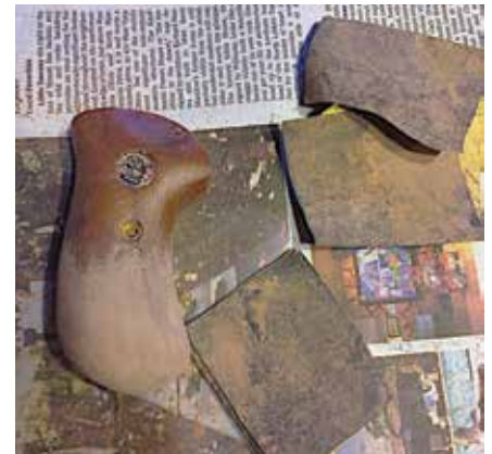
Some 220-grit sandpaper and a little elbow grease will clean up the cuts and contour the stocks to your liking.
