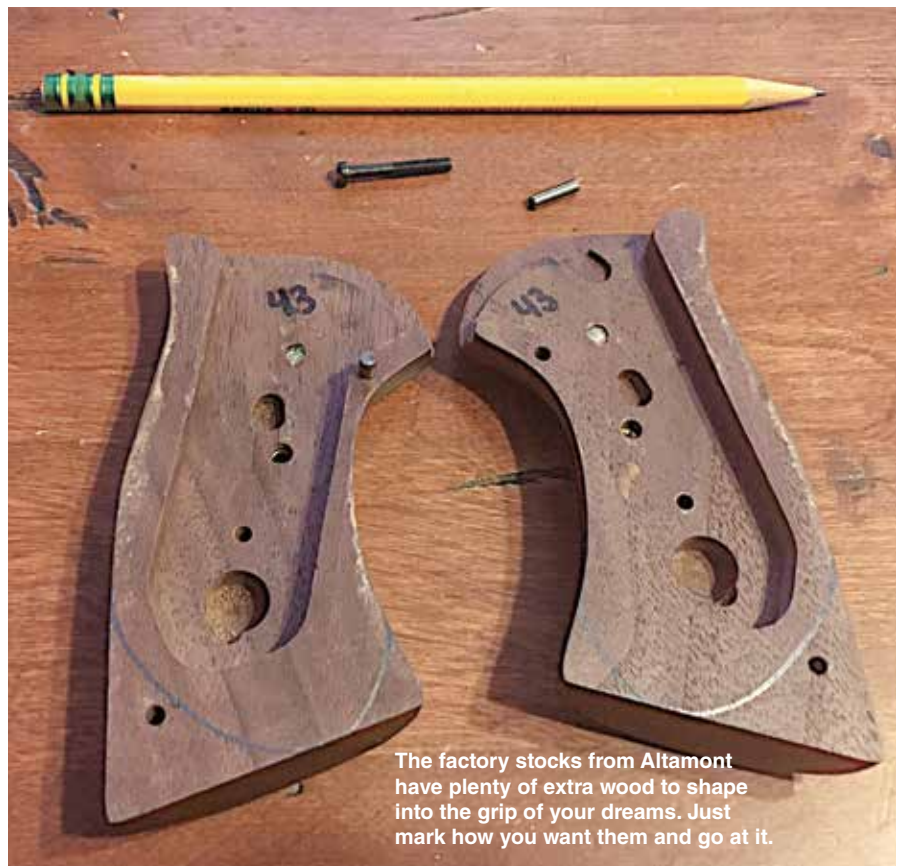
Some 220-grit sandpaper and a little elbow grease will clean up the cuts and contour the stocks to your liking.
