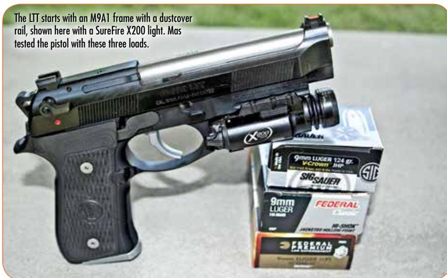
Langdon gives the Beretta improved checkering on the frame and an extended mag release.
