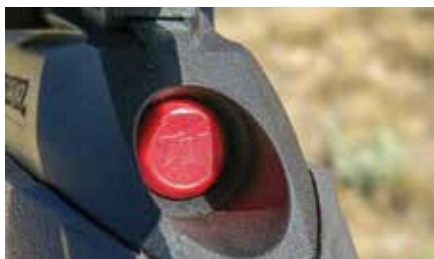
Pushing the red button enables the owner to remove the mechanics of the Wildcat for a thorough cleaning.
