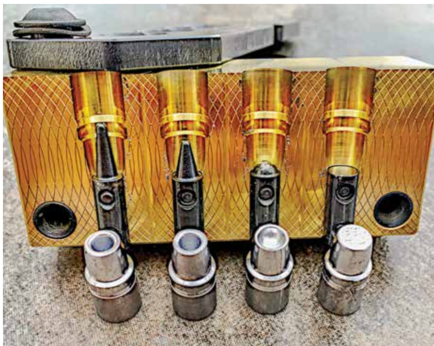
M-P Molds have different pins to allow different noses. Now it's socially acceptable to pick your nose and brag about the results!
