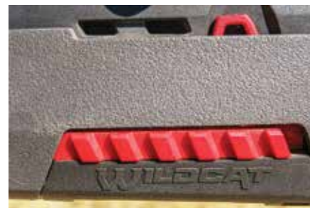
Sliding these grippy, red releases to the rear immediately ejects the magazine.
