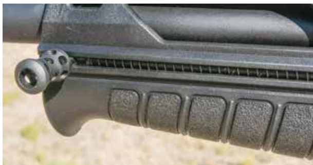
Bullpup guns are typically set-up for right-handed shooters with the charging handle placed on the left side.
