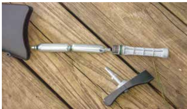
The two 12-gram CO 2 cartridges sit in the buttstock and power up using the integral wrench.
