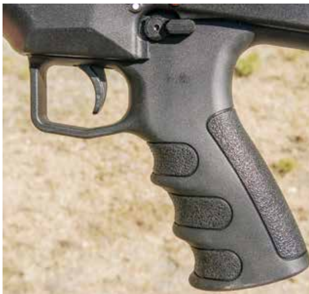
Because of the distance between the trigger and sear, bullpups typically have heavy trigger pulls. A vertical pistol grip with its improved trigger-finger position helps.
