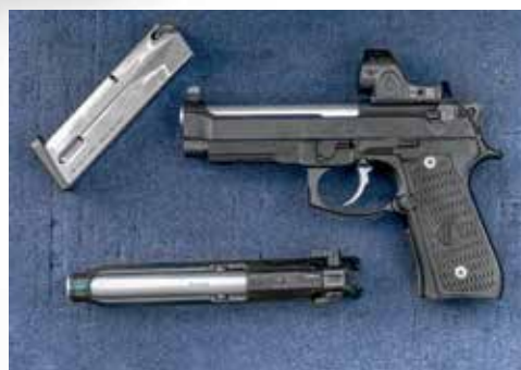
Langdon LTT Elite with RDO mount modification. Note how low the red dot sits on the slide.
