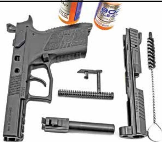
The slide lock lever doubles as the take-down control. Align the notches on the frame and push the lever through the frame.
