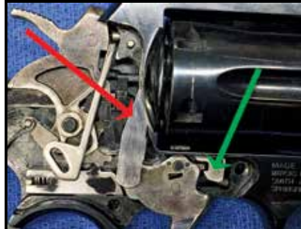
The “Hand” or “pawl” (red arrow) and the cylinder “stop” (green arrow) work together to move and lock the cylinder in place correcting “timing” so they both work together. When these wear, things can get “out of time.” Gun is a modern S&W Model 10.
