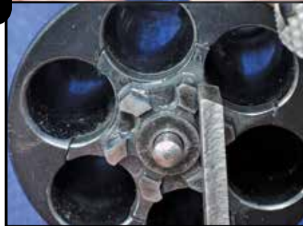
The “hand” (vertical metal piece) turns the cylinder by pushing on the ratchet cogs, finally bearing against the side of one cog. By then, the cylinder “stop” will have snicked into the proper notch in the cylinder, locking things in place.
