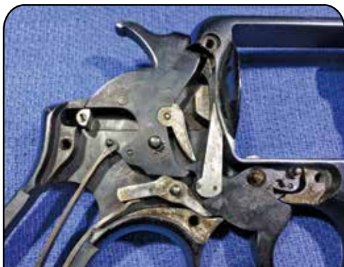
This 120 year old S&W Hand Ejector uses a “hand” and “stop” too, but the mechanics then were considerably different from a modern revolver. Roy was able to get this one “back in time” with some creative gunsmithing since there are no parts available.
