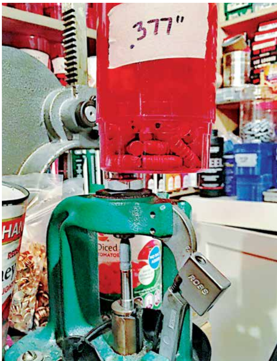
Tank sizes and applies gas checks with LEE push-thru sizing dies. He then sizes to 0.377" for best cast bullet accuracy in the .375 Winchester.
