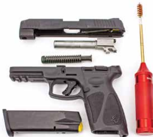
Disassembly is very similar to the GLOCK — there are slide removal tabs on each side of the frame and you need to pull the trigger before the slide will disengage.
