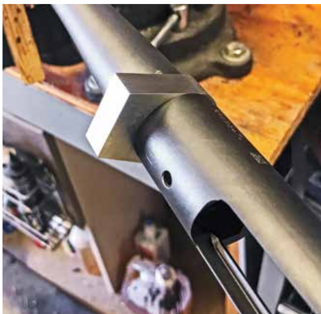
Tom replaced the stock Remington 700 3/16" recoil lug with a 3/8" thick heavy-duty one, surface-ground flat and parallel.
