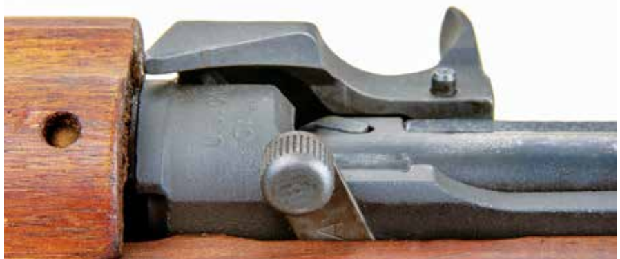
This small lever at the M2's left side determines semi-auto or full auto. It is forward in this photograph meaning the carbine is set for full auto.
