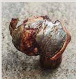
Close-up of a perfectly expanded Hornady RN 180-gr. .30 caliber slug recovered from a critter.
