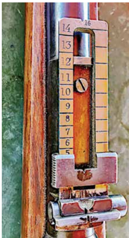
A close-up shot of the beautifully crafted rear ladder sight. It ranges all the way out to 1,600 meters.
