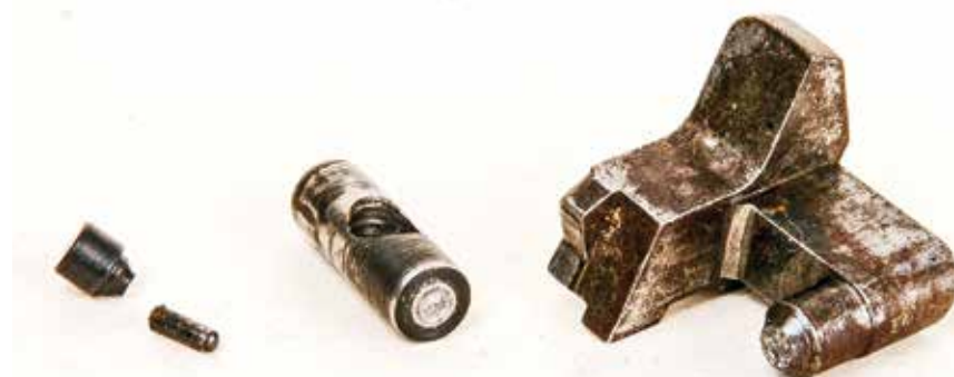
A tale of three pins: A broken firing pin for a modern Sharps Model 1874 replica (left), a Remington #1 "Rolling Block" showing a broken firing pin tip (middle) and an original Model 1874 transfer bar with the firing pin broken off.
