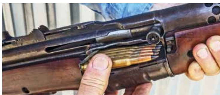
Here's how to load the Johnson via a 5-round stripper clip, plus you can also reload the rotary magazine with single rounds. Try this with your M1!
