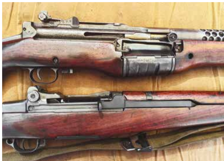
Comparison: the recoil-operated Johnson (top) and the gas-operated Garand (bottom). The Garand recoils slightly less and the safety is a bit quicker than the Johnson.
