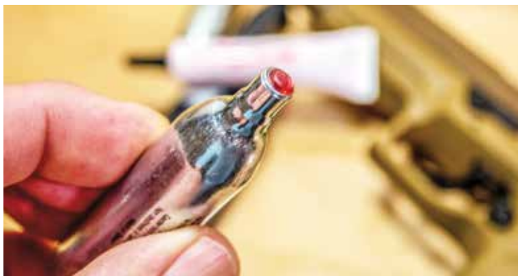
Maintaining a CO 2 airgun is easy — just add a drop of Pellgun oil to the top of each new CO 2 cylinder as you load it.
