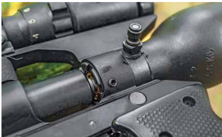
The Foster fitting where you connect an external air supply on a PCP is one place you definitely do not want to lubricate. Keep it dry and clean!
