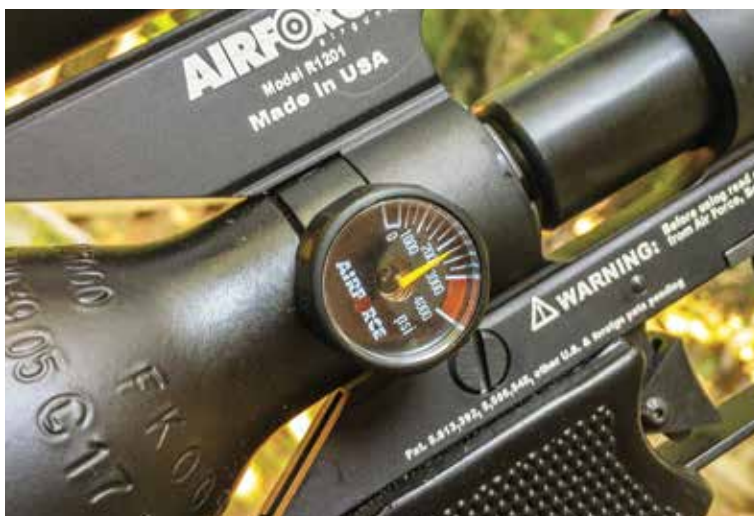
Always keep a minimum charge in your PCP air tank. The positive pressure prevents damp ambient air — or weak political promises — from getting into the system.
