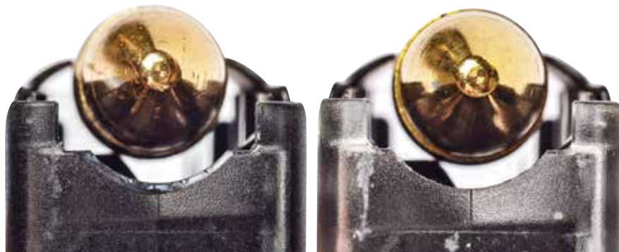
Loose lips, SOCOM ships: Wilson Combat opened their SOCOM-specific Lancer magazine (left) lips by 0.040" wider for reliability than the Lancer mag by Tromix.
