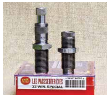
Essentials for loading the .32 Winchester Special include Lee Precision dies, as well as the Lee Universal Expander and Factory Crimp dies.
