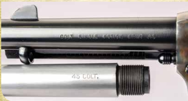
The gorgeous color-case-hardened hammer (above) now matches the frame. Caliber stamp on barrel (below) in the white during the Peacemaker Specialists remodeling compared with current style of caliber stamp.
