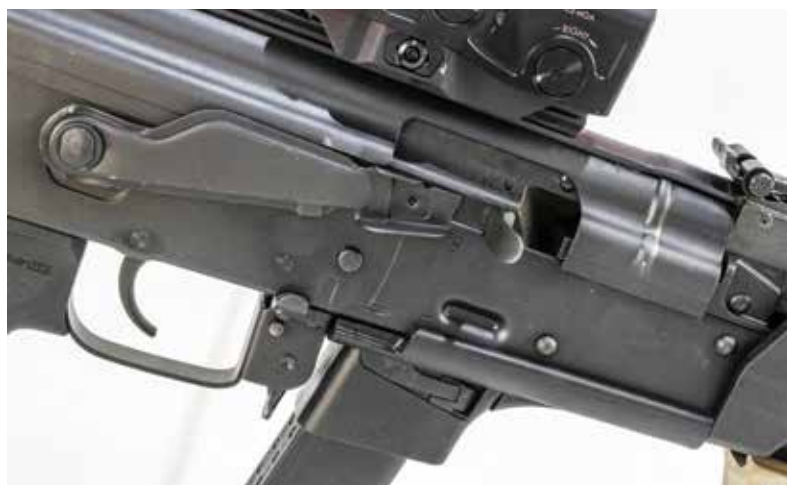
The action on the NAK9X is massively overbuilt. Note the bolt is fully closed but the angled cutout on the forward end makes it appear like it's cracked open.
