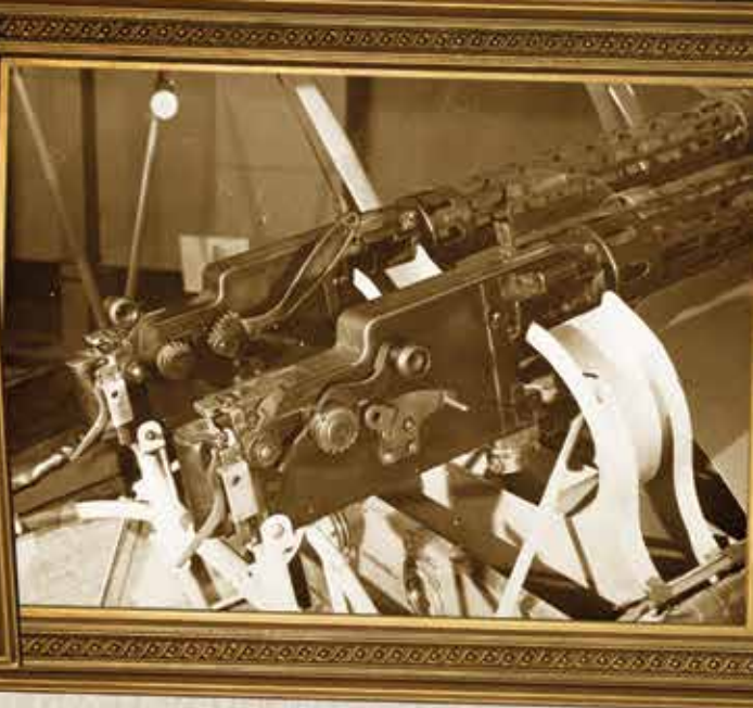
Twin 8mm Maxims, usually with 500 rounds each, became the standard German fighter armament in World War I.
