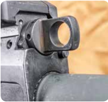
Four-position gas regulator allows firing under all conditions, even when fouled or wearing a snuffer on the business end.
