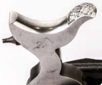
The checkering done on Duke's SAA hammer spur to match an 1880s hammer spur. Unfortunately, the firing pin cannot be changed to match an 1880s model.
