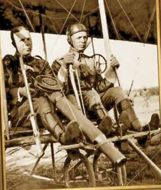
America's first mating of airplane and machine gun occurred in 1912 when three army pilots took aloft a Lewis Gun for three days of tests in a Wright Flyer.
