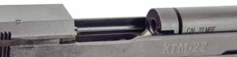
The barrel, shroud, recoil guide rod and spring (above) are noticeably different from the 1911. The end of the recoil guide rod should be frequently checked for tightness. The barrel and barrel shroud (below) are different than a standard 1911's with a gap between barrel and shroud to release gas pressure.
