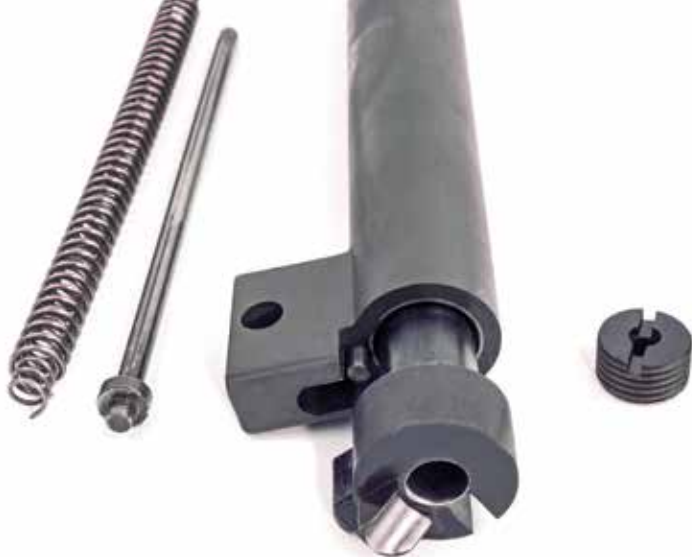
The barrel, shroud, recoil guide rod and spring (above) are noticeably different from the 1911. The end of the recoil guide rod should be frequently checked for tightness. The barrel and barrel shroud (below) are different than a standard 1911's with a gap between barrel and shroud to release gas pressure.
