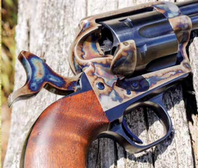
The gorgeous color-case-hardened hammer (above) now matches the frame. Caliber stamp on barrel (below) in the white during the Peacemaker Specialists remodeling compared with current style of caliber stamp.
