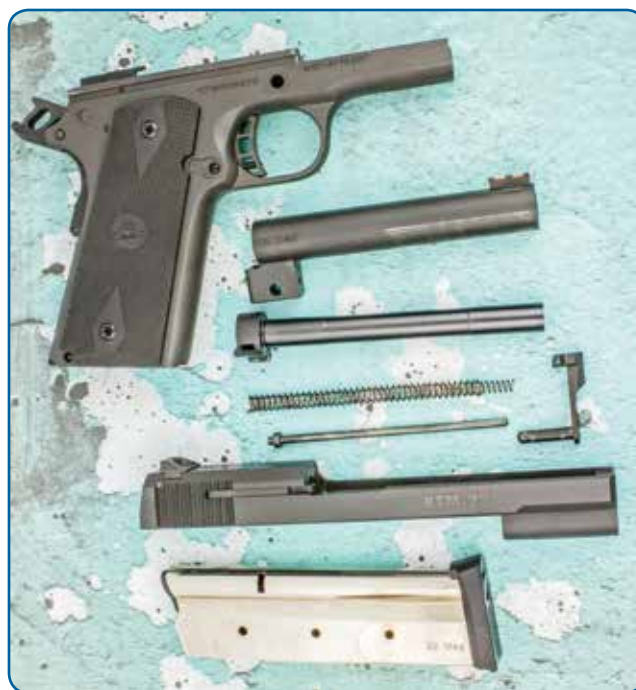
Disassembly is almost classic 1911 but with few extra parts.
