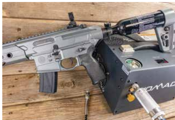
You can fill its 3,000 psi air cylinder with a high-pressure hand pump but this Nomad portable compressor from Air Venturi makes the job much easier.
