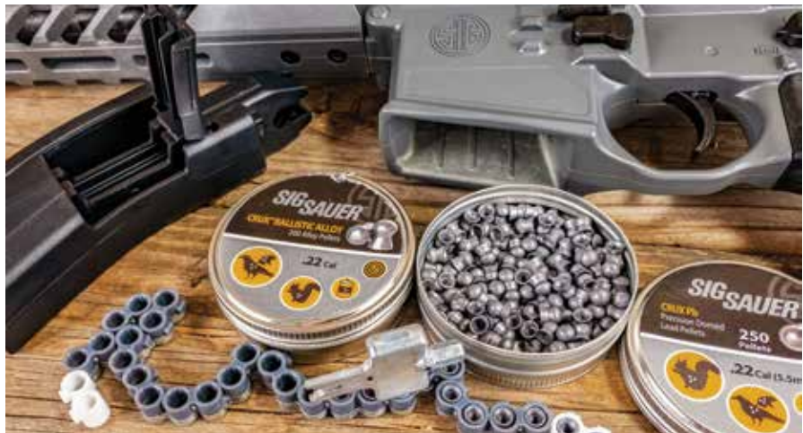
The magazine drops just like the centerfire version but runs off an internal 30-pellet belt.
