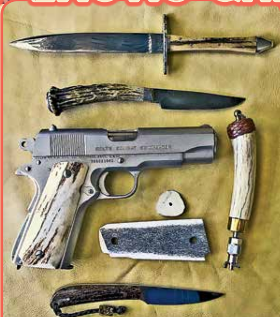
Top to bottom: Stag, deer antler, elk 1911 scales and kudu horn. The weird stuff in the middle is a cross section of axis antler showing no pith at all, the back of an elk 1911 scale showing pith and good wall depth and one of Karla's stitching groove tools made with a deer antler stabilized with cyanoacrylate glue after severe exposure to the seasons in the field.
