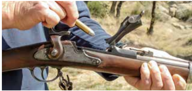
To reduce costs, Springfield used Civil War era locks on the new Trapdoors (left). Allin's ingenious cartridge conversion soldiered on until the adoption of the Krag (right).
