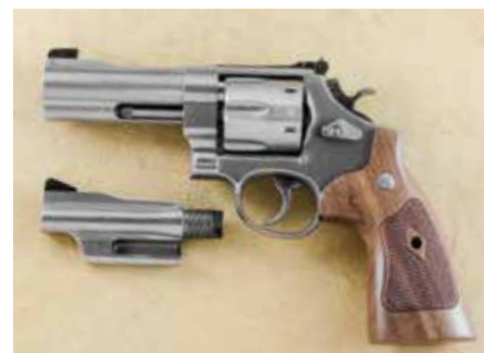
The second Mountain Gun came back from S&W with a heavy under-lug barrel and new S&W target stocks.
