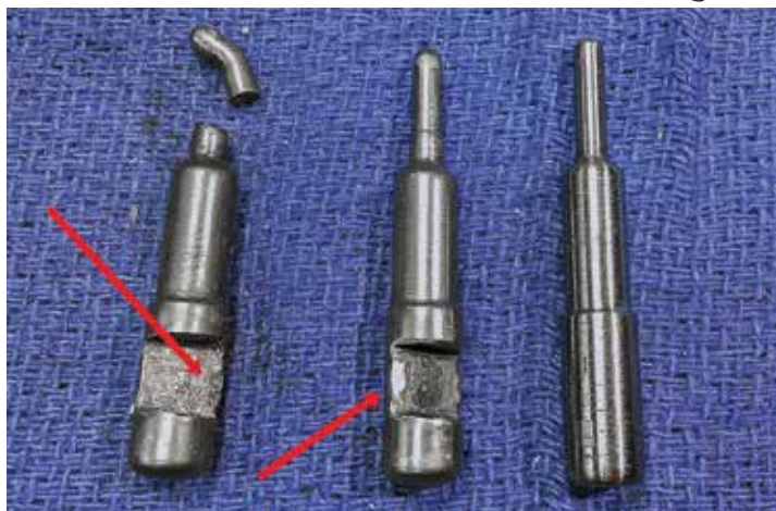
(L-R) The broken pin, the unbroken pin and the "made from lag-screw" rough version. Notice the peening and wear on the old pins due to soft steel.
