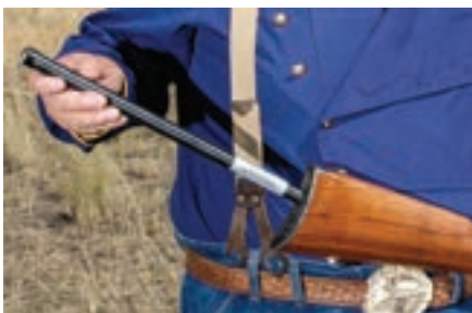
The system for loading the Spencer is akin to how some .22 rimfires are loaded still.
