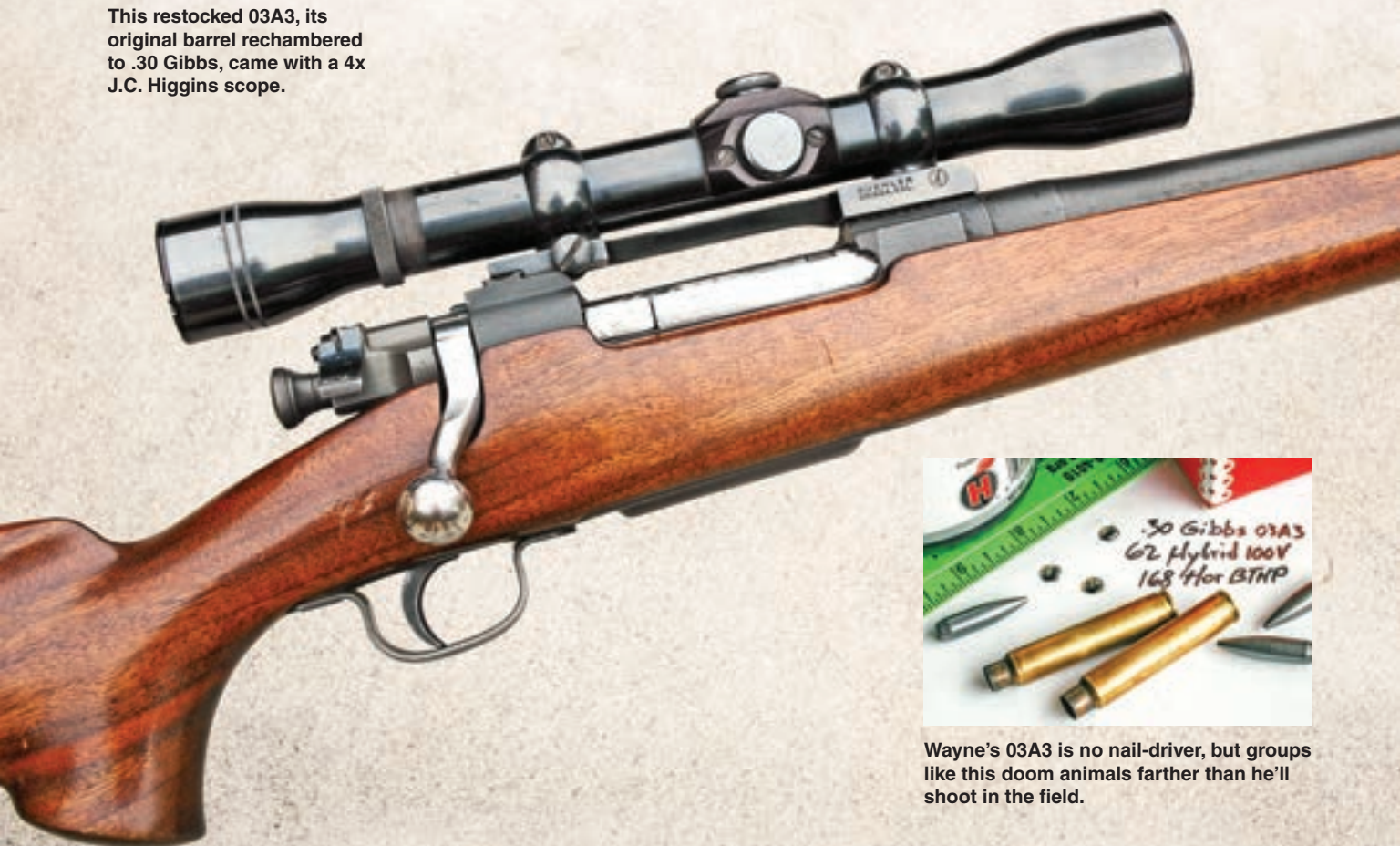
Building a .30 Gibbs from .30-06 brass: Neck up to .33 or .35, form a new shoulder with a Gibbs die, fire-form.
