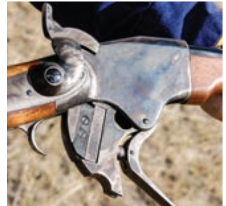
Taylor & Company's Model 1865 Spencer with lever down and breechblock lowered.
