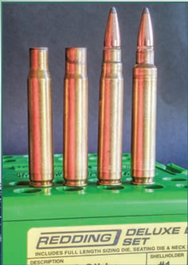
Building a .30 Gibbs from .30-06 brass: Neck up to .33 or .35, form a new shoulder with a Gibbs die, fire-form.
