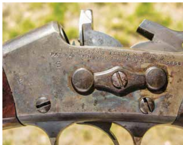
The rolling-block action (above) is simple, strong and fast to operate. The frames were color casehardened (below). "P S" stands for "Proved Stickney," in reference to Inspector Curtis R. Stickney.
