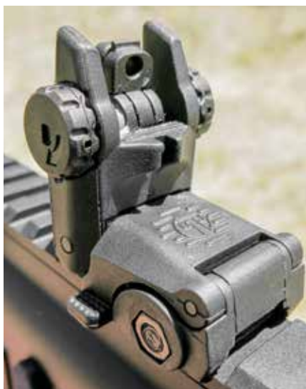
The Picatinny rail of the Elite carries a set of fully adjustable flip-up sights.
