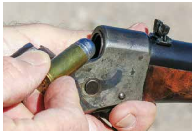
The rolling-block action (above) is simple, strong and fast to operate. The frames were color casehardened (below). "P S" stands for "Proved Stickney," in reference to Inspector Curtis R. Stickney.
