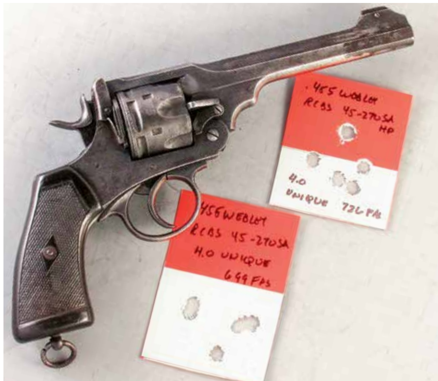
These targets (above) were fired with John's S&W 2nd Model .455 using loads approaching .45 Colt performance with 5.0 grains of Unique. Standard .455 level groups (below) were fired in John's Mark VI at 20 yards. Not bad for an old Brit warhorse!
