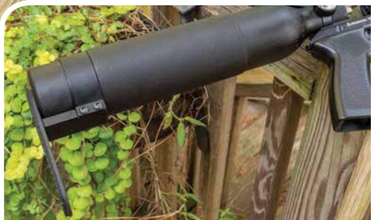
The large air reservoir of the AirForce Condor (above) performs double duty as a stock. Total efficiency! These are .25-caliber 48-gr. HP bullets from Hunters Supply (left). If you want heavier, you can order varieties up to 105 grains.
