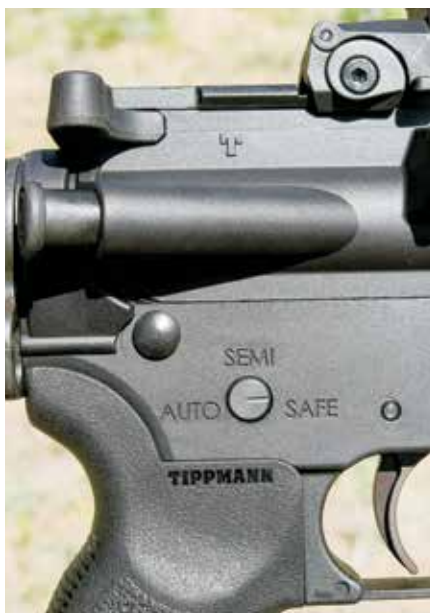
A quality AR clone should have functional controls in the right places. Holt was particularly impressed with the working forward assist.
