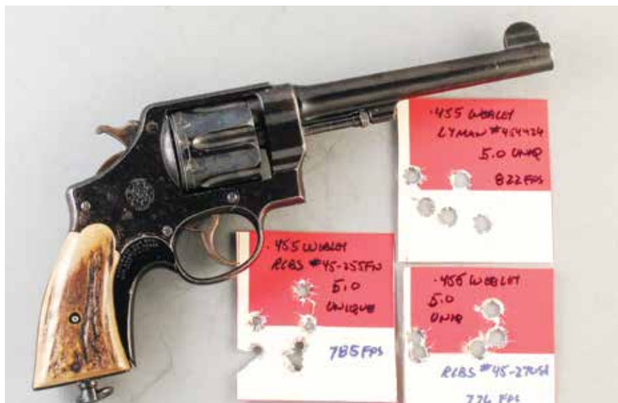
These targets (above) were fired with John's S&W 2nd Model .455 using loads approaching .45 Colt performance with 5.0 grains of Unique. Standard .455 level groups (below) were fired in John's Mark VI at 20 yards. Not bad for an old Brit warhorse!
