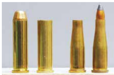
The .357 Magnum case is the parent case for the .22 Jet.
