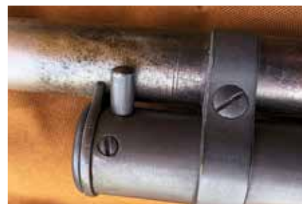
The takedown pin is located at the end of the magazine.
