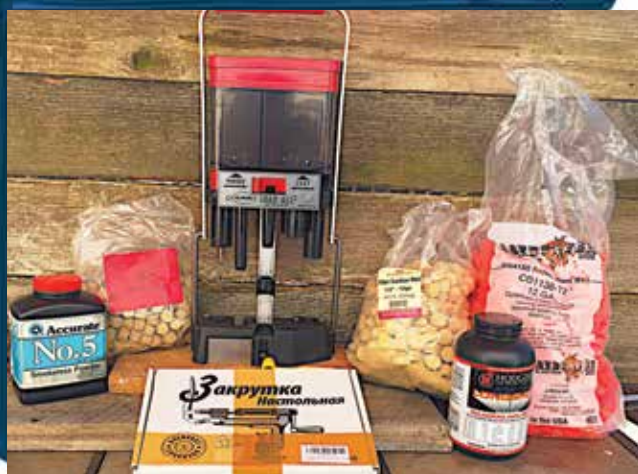
The Lee Load All II makes loading simple and economical. Here it's flanked by some of the other components Tank used for his handloaded slug rounds.
