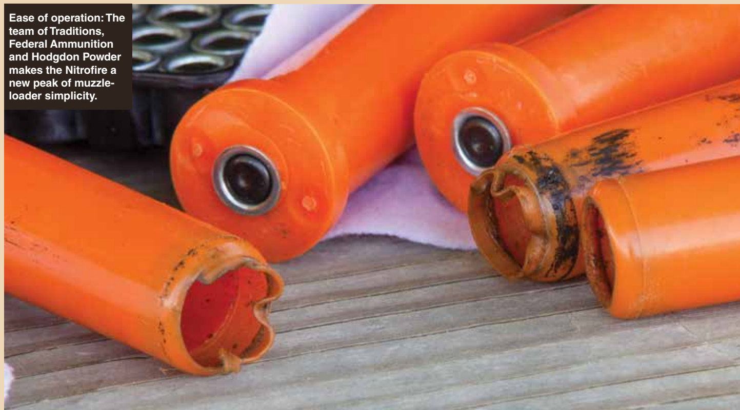
Standard #209 shotgun primers ignite the Hodgdon Triple 8 black powder substitute.
