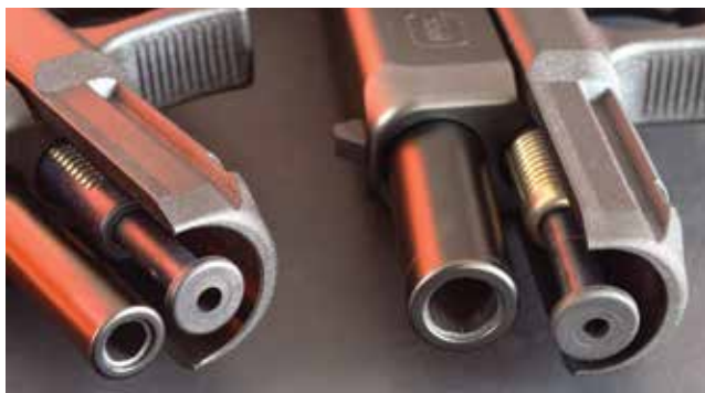
The G44 (above, left) is clearly of G19 lineage, but its "hybrid" slide keeps loaded weight to 16 oz.! The G44 ships with two 10-shot magazines (below), nearly identical in outside dimensions to the G19.
