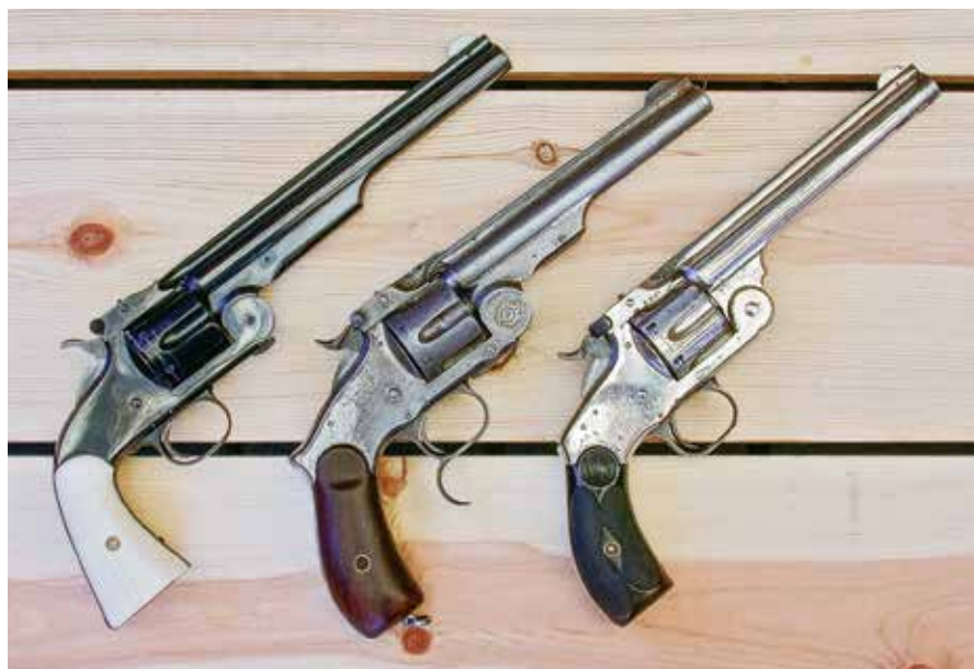
The Smith & Wesson evolution (left to right) — .44 American, .44 Model #3 Russian and New Model #3 .44 Russian. The first Russian is notable for its humpback design and trigger guard spur.
