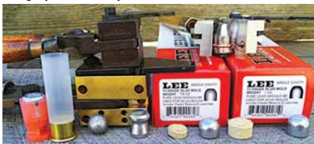
Here's a close-up of the molds and projectiles Tank cast, loaded and shot. Molds from Lyman, Lee and MP-Molds worked exceptionally.
