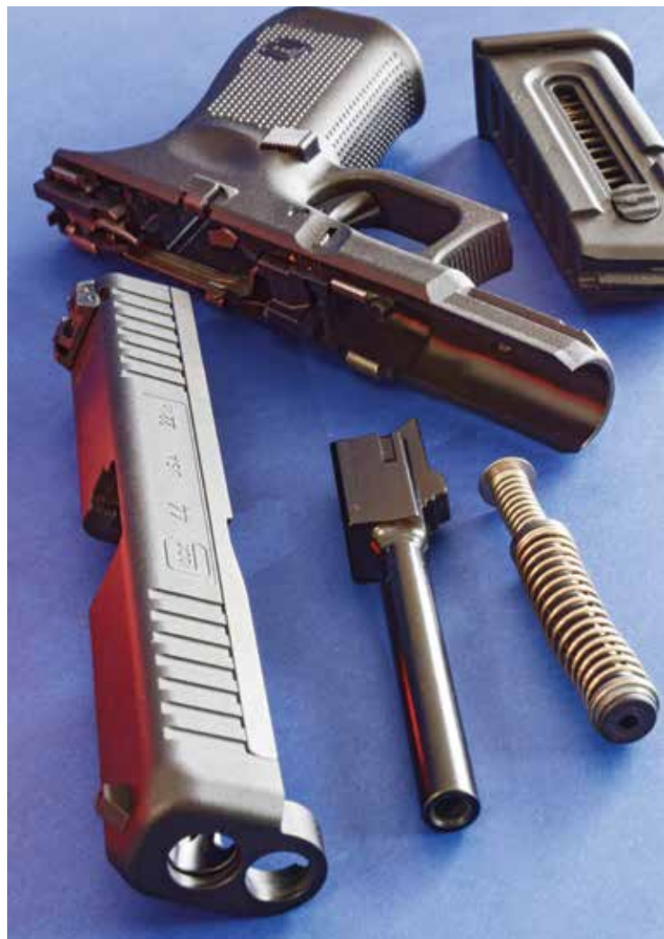
Field-stripping a G44 is a cinch without tools. A threaded, suppressor-ready barrel is sold separately. "Okay. I pulled one," Wayne said, but five (below) of the G44's first six shots over bags at 25 yards nipped into 1.3".
