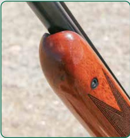
The Browning Double Automatic was the only semi auto shotgun made with no fore-end cap until the recent Browning Maxus, giving it a sleek profile.
