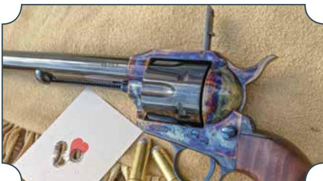
The Standard Target Model features the unusual flip-up elevated rear sight, modified hammer screw for mounting a shoulder stock and rifle-style front sight like the original.
