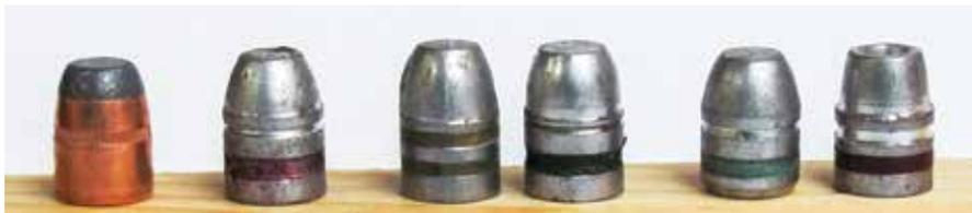
Cast bullets in the 200-gr. weight range compared to a 200-gr. jacketed .44 Magnum bullet (above, left). For an easy shooting .44 WCF levergun/sixgun combination, John matches up an Uberti Model 1873 with a Colt Single Action.
