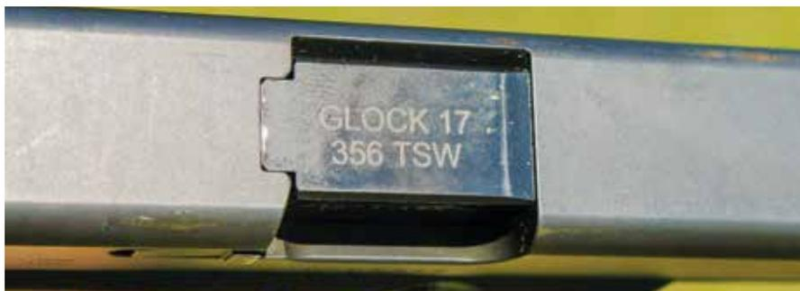
Scott Sullivan's drop-in .356 TSW conversion barrel in GLOCK 17. The kits currently only work in GEN 3-4 guns.
