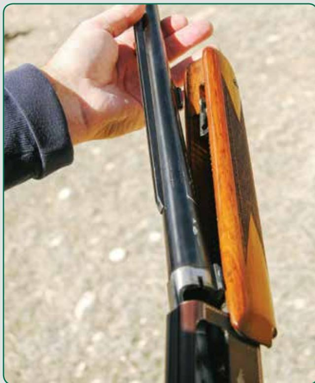
Barrel removal can be accomplished in a matter of seconds (above), though not many understand why “speed re-barreling” was touted as a critical benefit by Browning. Since the gun has no magazine, the second shot rides on the shell carrier (below). Glancing at the loading port tells the shooter immediately if the gun is fully charged.
