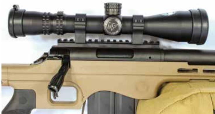
A NightForce NXS 2.5-10x42 scope (above) was mounted on the LRR in Warne horizontal rings. Length of pull and comb height (below) may be adjusted via large dials on the aluminum chassis. It also sports plenty of fore-end slots for accessories.
