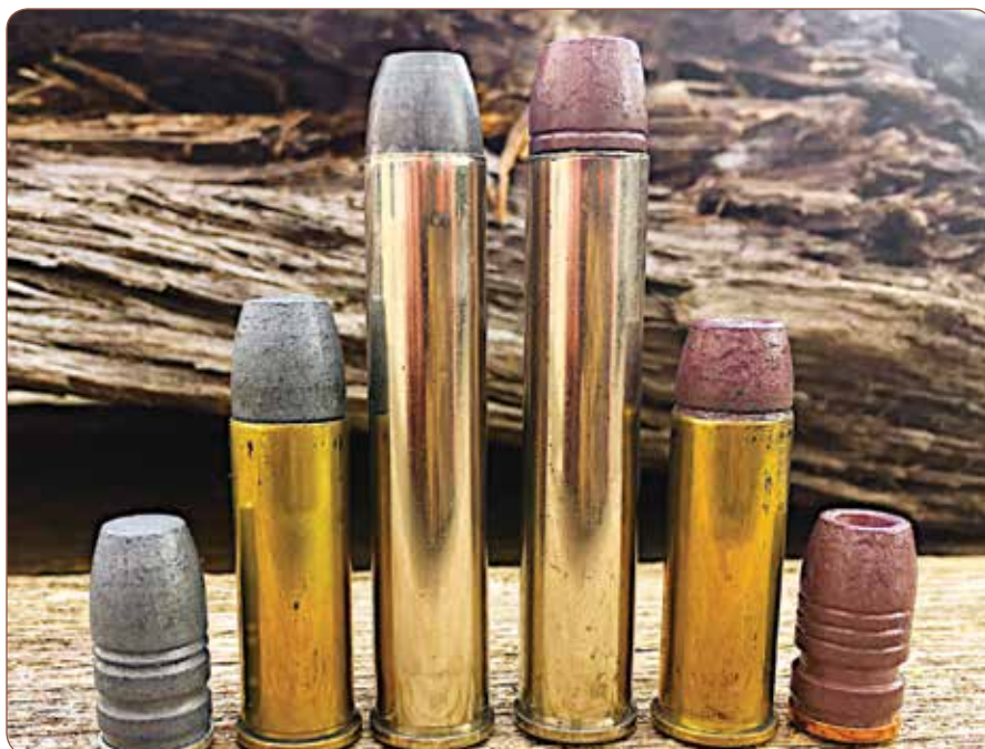
Tank's favorite molds for the .444 Marlin — LBT 330-grain LFNDCGC at left and MP Molds 300-grain HP on right. Both molds work wonderfully in .44 Mag too!
