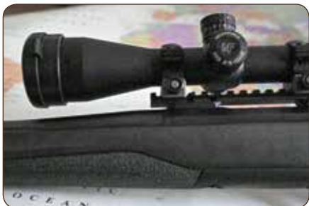
Browning X-Bolt Composite Stalker has a short bolt lift with plenty of hand clearance between bolt and scope for Dave's choice of a Nightforce 2.5-10x42 scope on a 20 moa Talley rail.
