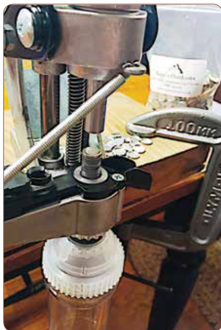
The LEE APP press is a fast, easy, fun way of sizing and crimping gas checks onto your cast slugs. Remember, 0.432" is the way to go for top accuracy.
