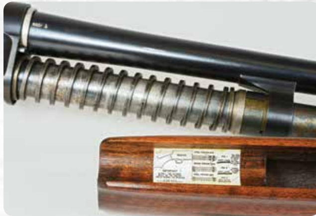
In the A5/M11, Browning incorporated a clever series of fouling-insensitive friction rings around the magazine tube to adjust the gun for differing loads.
