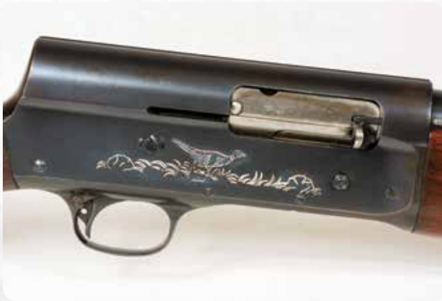
The Model 11's barrel, like the A5, has a distinctive "Hump-back" shape. Due to wartime exigencies, many military shotguns still had a hunting scene stamped on the receiver.
