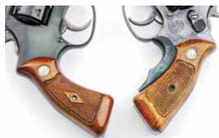
Tyler-T grip adapter on J-Frame S&W (right) greatly improved "fit" over standard stocks (above, left). This shooter finds trigger reach optimal on his Sarsilmaz SAR 9 (below).
