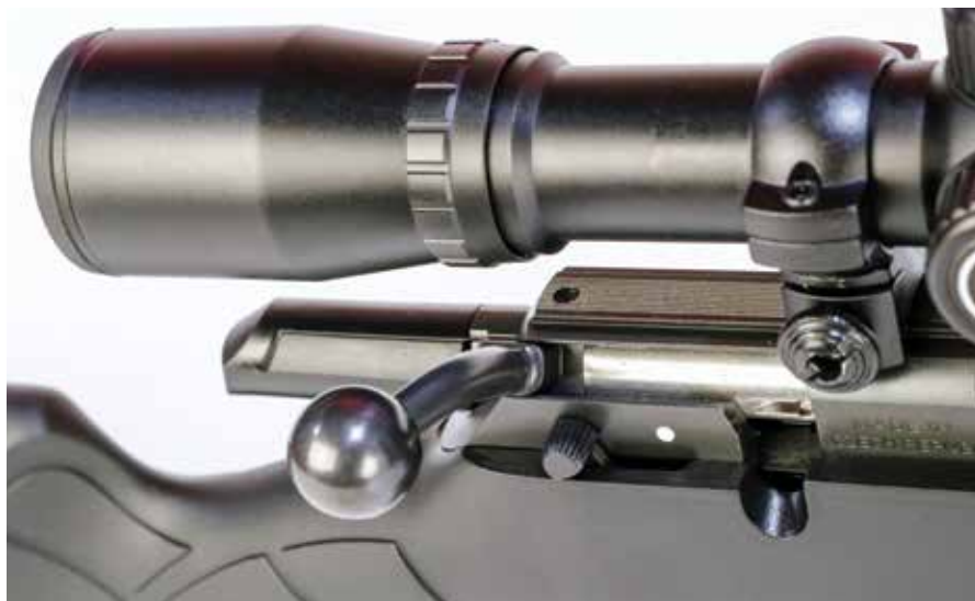
The 60-degree bolt throw offers a rapid rate of fire and clearance for a scope.
