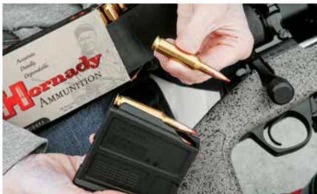
When choosing a load for a re-barreling/re-chambering project, make sure the box accepts loaded rounds!
