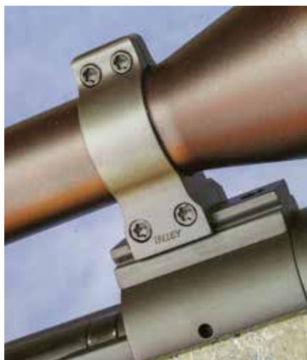
Leave at least 1/8" between rings and scope tube flares and junctures. Snug screws alternately.
