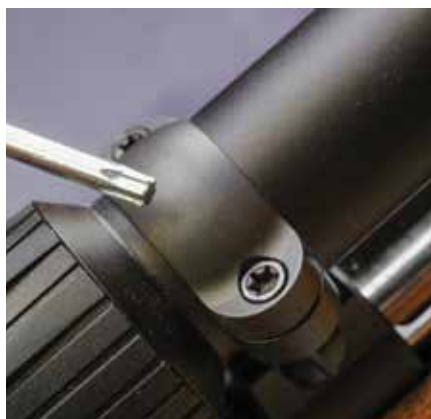
Torx wrenches are kind to screws. Use the short end for leverage on rings. No more torque needed.
