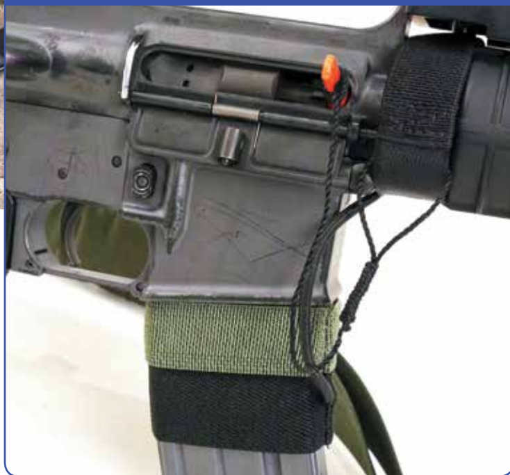
Short and lightweight, the IDF Mekut'zar carbine (left) is better rigged for combat than the old U.S. M16s and much easier to tote all day. A loaded magazine (below) is secured to the rifle via this nifty elastic rig from Zahal.org.
