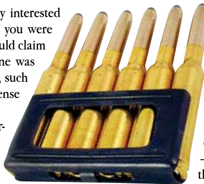
The 6-round Mannlicher clip made from brass or soft steel. They were easier to load than stripper clips and gave the Italians a slight ammo superiority, but also rendered the rifle a single shot if no clips were available.
