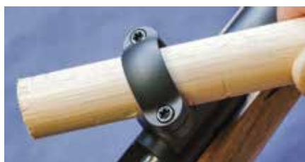
Turn dovetail rings in with a 1" dowel — not the scope — lest you bend it or damage it internally.
