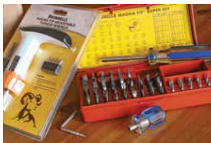
Use hard, hollow-ground bits to protect screw heads. A torque wrench and screwdriver set give you mar-free scope mounting and a secure optic.
