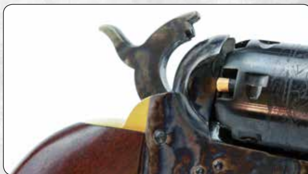
When fired as a muzzleloader, the 1851 Navy revolver (above) depends upon percussion caps pressed on the nipple for each chamber to ignite the black powder. When equipped with a conversion cylinder, each chamber has its own firing pin (below).
