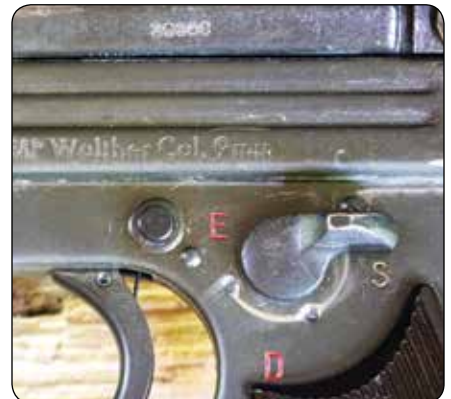
The fire selector rotates through 180 degrees like an M4 but the semi and full auto positions are reversed.
