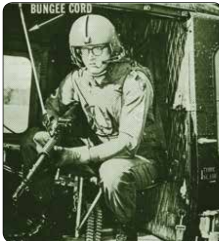
Early door guns were simply ground guns suspended via bungee cords from the ceiling of the aircraft.
