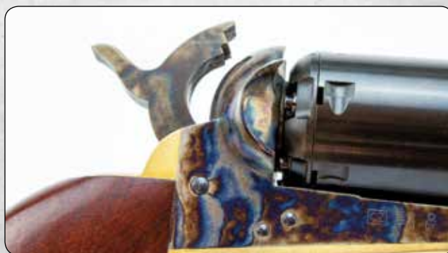
When fired as a muzzleloader, the 1851 Navy revolver (above) depends upon percussion caps pressed on the nipple for each chamber to ignite the black powder. When equipped with a conversion cylinder, each chamber has its own firing pin (below).
