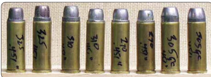
John makes up dummy loads using available cast bullets (above) to make sure they will feed and chamber through levergun actions. Cast bullets in both plain-based and gas check versions (below) are available from 260 grains to 325 grains.
