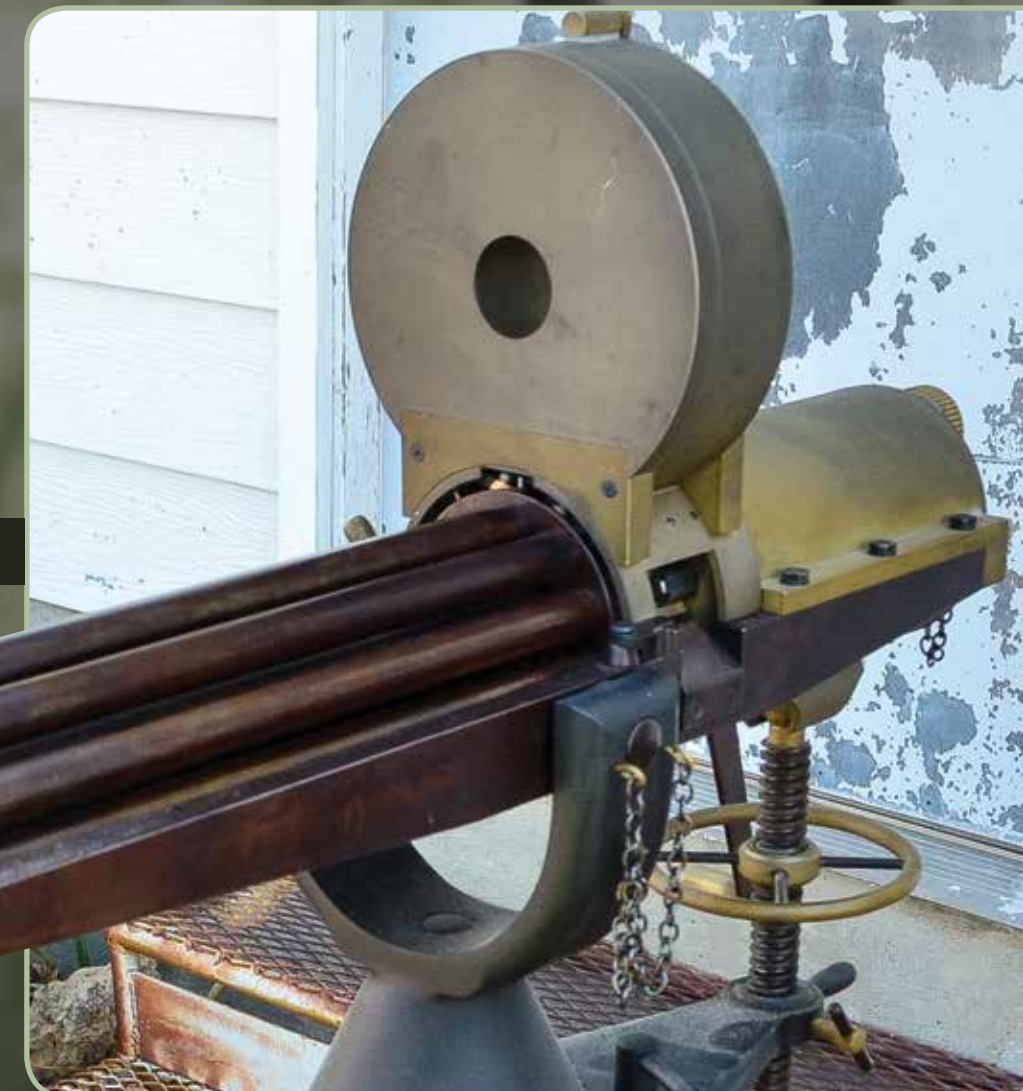
The hand-built elevation and traverse mechanism allows aiming and closely echoes the original design. Left, the hand-built .22 LR Gatling gun built by farmer, gunsmith and machinist Kenneth Hower. Below a closeup of the breach of the .22 LR Hower Gatling gun. All parts were hand-fabricated from blueprints, which turned out wrong in many cases!
