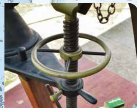
The hand-built elevation and traverse mechanism allows aiming and closely echoes the original design. Left, the hand-built .22 LR Gatling gun built by farmer, gunsmith and machinist Kenneth Hower. Below a closeup of the breach of the .22 LR Hower Gatling gun. All parts were hand-fabricated from blueprints, which turned out wrong in many cases!
