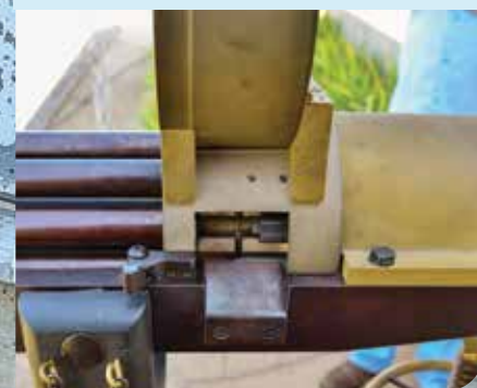
The hand-built elevation and traverse mechanism allows aiming and closely echoes the original design. Left, the hand-built .22 LR Gatling gun built by farmer, gunsmith and machinist Kenneth Hower. Below a closeup of the breach of the .22 LR Hower Gatling gun. All parts were hand-fabricated from blueprints, which turned out wrong in many cases!
