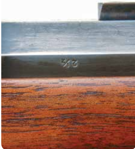
The Sharps factory-marked chamberings by case length and not by powder capacity. This one was a .40-70 Sharps Straight.
