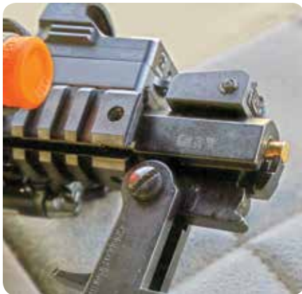
Rotating the barrel about 90 degrees lets the extractor lift the fired case from the chamber so it can be easily removed by hand by the shooter.
