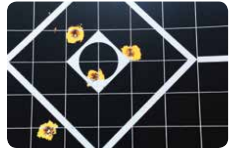
One hundred yards scoped: Four of five are within 3", a pretty solid performance for a G/K43 using a standard service round equivalent.
