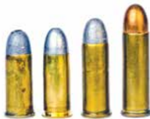
Bottom: From left: original Japanese 9mm rimmed cartridge, Duke's handload with Buffalo Arms brass and Oregon Trail 147-grain bullets, U.S. .38 Long Colt military round, and a U.S. .38 Special military round. Note the FMJ bullet.
