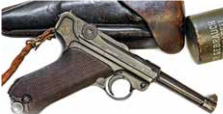
Georg Luger designed this pistol to fire a necked-down cartridge. When the German military wanted a larger bore, Luger expanded it to 9mm.
