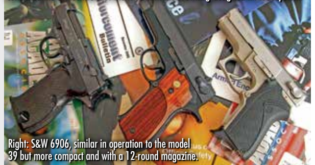
Evolution of 9x19 pistols — Left: Walther designed P-38; Center: S&W model 39 combined the DA lockwork of the P-38 with the Browning-designed tilt-lock system.
