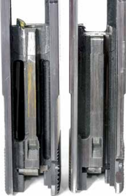
Left: Centerfire slide from SVI/Infinity (right) shown with the matching one Jeremy converted to a .22 (left). Notice the longer breechface and the lightening cuts near the disconnect. It's some of his first machine work and not pretty, but it functions.
