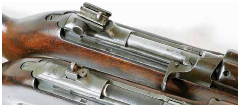
The top rifle sports a round bolt, an adjustable rear sight and the four-rivet hand-guard characteristic of late-model guns. The early run rifle on the bottom has a simple flip sight, a two-rivet handguard and a flat bolt. Normal people don't care, but carbine nerds sure do.
