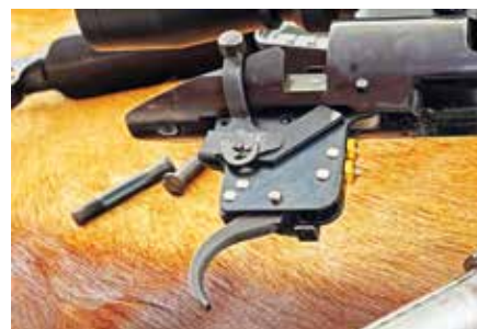
Dave bought this used early '70s-era Remington 700 in .243 but a previous owner had fiddled with the adjustment screws of the trigger to the point it was unsafe. A Shilen trigger solved the problem.
