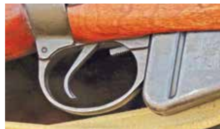
The Lee Enfield service rifle in its various models had a typical military two-stage pull — a long first-stage pull to a positive stop, followed by a short, crisp second stage.
