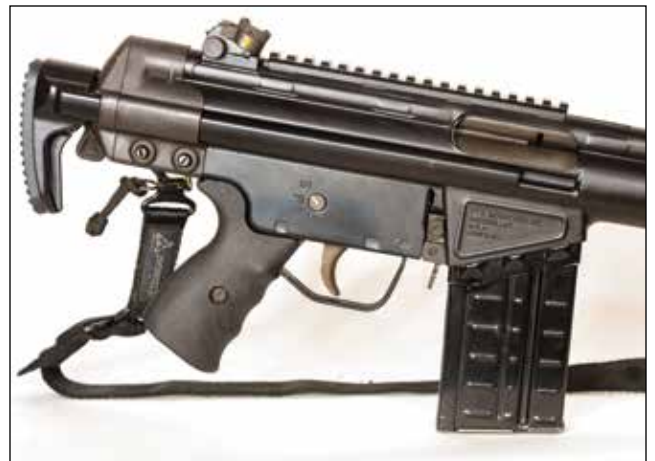
The 16" PTR91 has been modified with a collapsible A3 buttstock, KeyMod fore end, 900-lumen Crimson Trace light, PWS muzzle device and Trijicon tritium sights, Magpul sling and an extended cocking handle.
