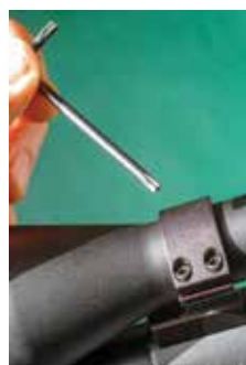
Before zeroing or checking zero, snug screws. Any change in tension could well affect point of impact.
