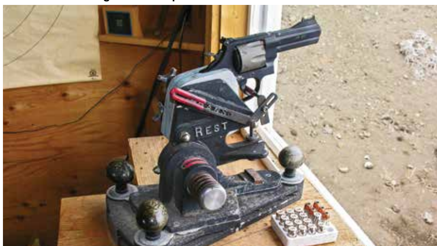
Duke shown test-firing an S&W Model 24 .44 Special mounted on a Ransom Pistol Machine Rest. This close-up shows the mounting arrangement of Duke’s Ransom Rest in his shooting house and particulars of the rest itself.
