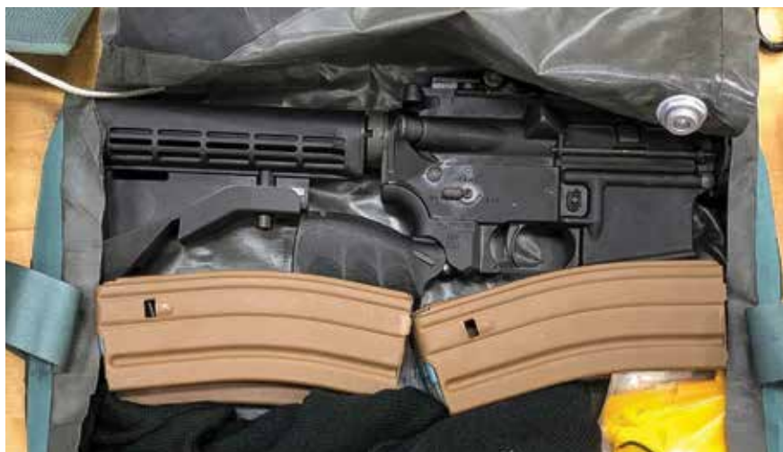
The Cry Havoc system allows the rifle to be stored in a backpack (above) yet retains zero when reassembled. The GAU-5A (below) is a selective-fire takedown survival arm carried in all USAF combat aircraft in the ejection seat survival kit. It uses the Cry Havoc QRB kit. Photo: USAF
