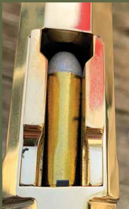
Loading is easy. Simply push the magazine follower to the top and twist the top 5" of the barrel/magazine clockwise. Then drop your cartridges into the magazine. Below is a cartridge on the elevator, ready to be chambered. Cycling is as smooth as could be.
