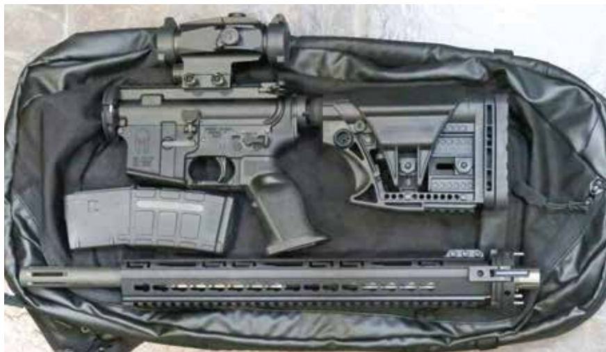
The Cry Havoc system allows the rifle to be stored in a backpack (above) yet retains zero when reassembled. The GAU-5A (below) is a selective-fire takedown survival arm carried in all USAF combat aircraft in the ejection seat survival kit. It uses the Cry Havoc QRB kit. Photo: USAF
