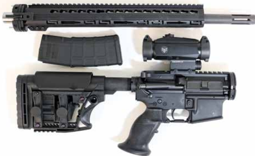
The Cry Havoc Tactical QRB kit produces a takedown rifle that breaks down and assembles in seconds yet reliably retains its zero.
