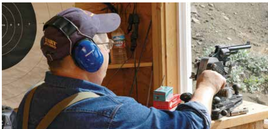
Duke shown test-firing an S&W Model 24 .44 Special mounted on a Ransom Pistol Machine Rest. This close-up shows the mounting arrangement of Duke’s Ransom Rest in his shooting house and particulars of the rest itself.
