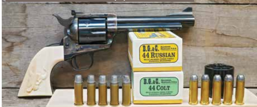
The versatility of the 5-1/2" .44 Special New Frontier — the original cylinder not only handles .44 Specials but .44 Colts and .44 Russians while the auxiliary cylinder is for .44-40s.
