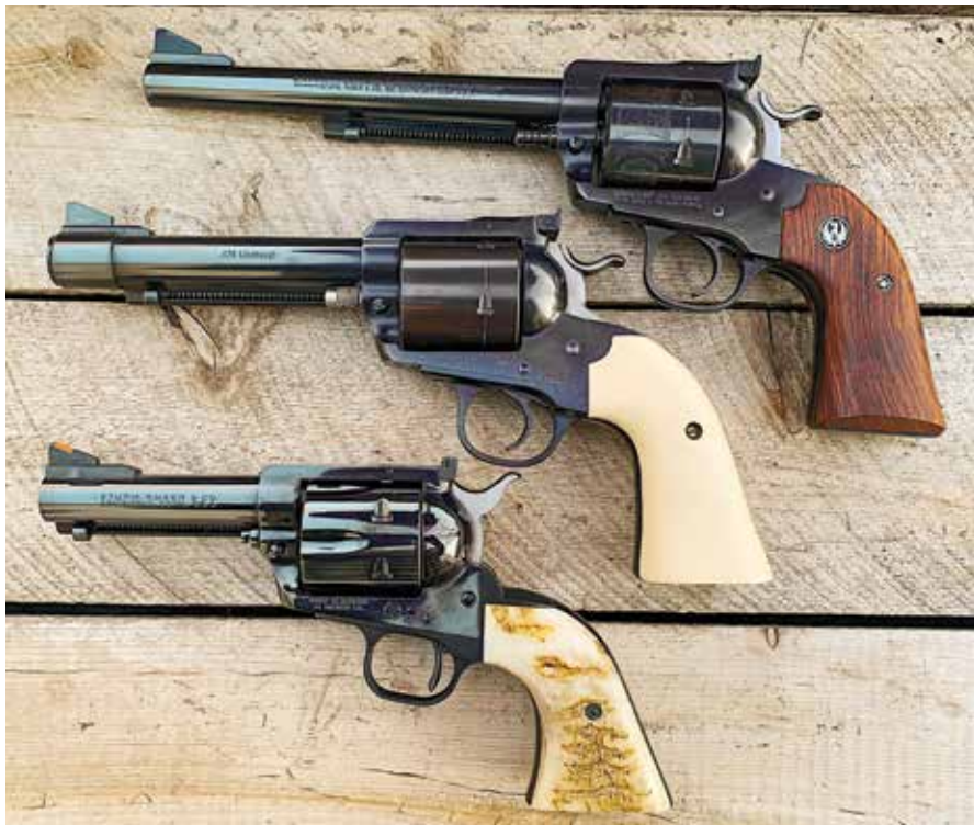
The top gun was the first Tank worked over by honing cylinder throats, replacing a base-pin and trigger job. Middle gun is a simply perfect John Linebaugh custom; bottom, a Ken Kelly of Mag-na-port custom.
