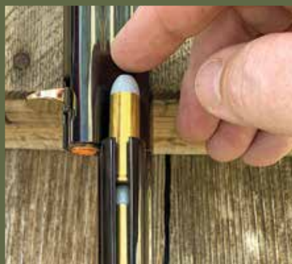
Loading is easy. Simply push the magazine follower to the top and twist the top 5" of the barrel/magazine clockwise. Then drop your cartridges into the magazine. Below is a cartridge on the elevator, ready to be chambered. Cycling is as smooth as could be.
