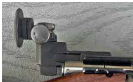
Vintage Redfield aperture sights — front and rear — establish the Model 75's paper-punching credibility.
