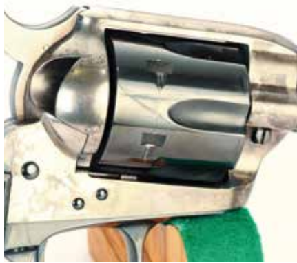
Close up of Duke's 3rd Generation Colt SAA .32-20 (above) with its new color case hardening. Close up of the same gun (below) with its frame colors removed.
