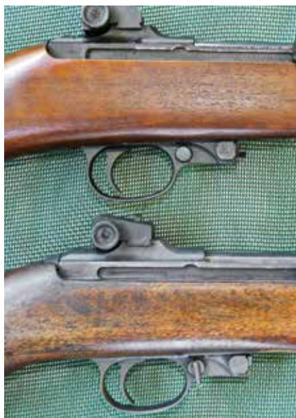
Top carbine (above) has M2 mag catch for use with 30-round magazines and will hold the bolt back after last shot is fired. M1 on top (below) uses button-type safety. A lever safety replaced the button on later versions. Both are shown in the "safe" position.
