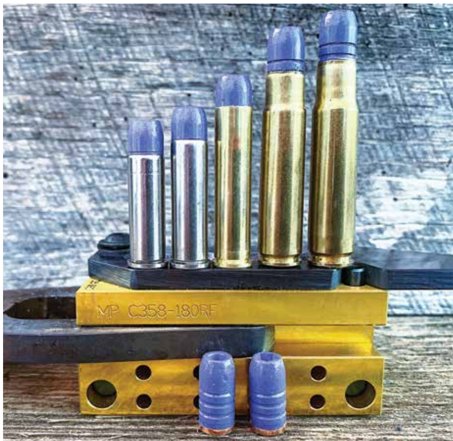
MP-Molds 358-180RFGC is very versatile, capable of loading (left to right) .38 Special, .357 Magnum, .357 Maximum, .35 Remington and .358 Winchester, to name a few.
