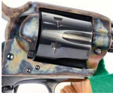
Close up of Duke's 3rd Generation Colt SAA .32-20 (above) with its new color case hardening. Close up of the same gun (below) with its frame colors removed.
