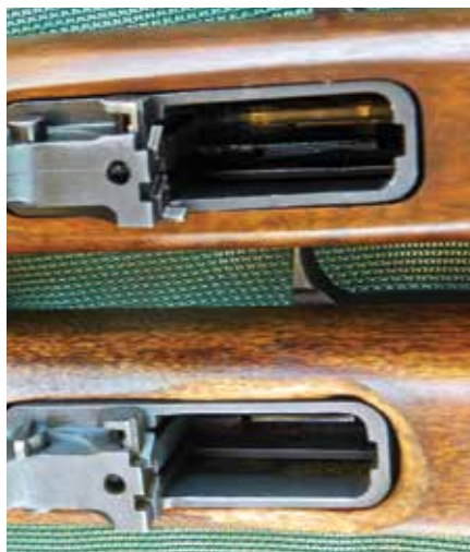
Top carbine (above) has M2 mag catch for use with 30-round magazines and will hold the bolt back after last shot is fired. M1 on top (below) uses button-type safety. A lever safety replaced the button on later versions. Both are shown in the "safe" position.
