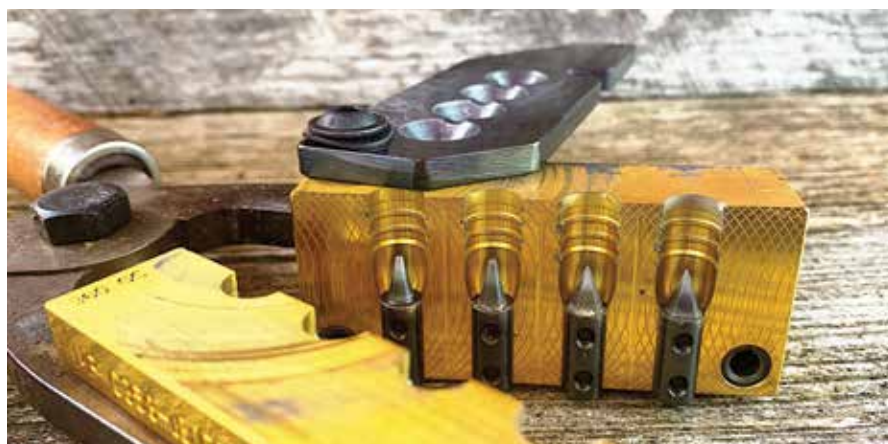
Shown are the insert pins allowing for different hollow points. A solid option is also possible.
