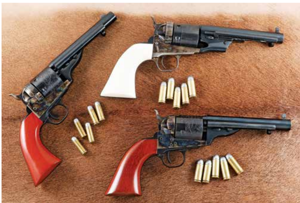
Here we have all three cartridge-firing Colts based on the 1860 Armory. From the left clockwise, conversions are the Richards-Mason, Richards and 1871-72 Open-Top.
