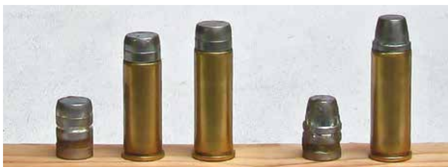
Above, Alliant Dot powders performed well in the 4" pre-29 and the 4" stainless steel .45 Auto Rim and .45 Colt. Custom stocks are by BluMagnum. Below, both the .44 Special and .44 Magnum loads were assembled with Accurate Molds #43-249 while the .45 Colt uses the Lyman #452424.
