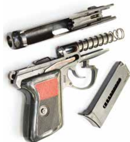
This is a standard P-64 of 1970s manufacture (above) showing the improved, triangular shaped hammer. Note the distinctive humped back and the windage adjustable rear sight. The P-64 pistol operates and field strips (below) like a Walther PPK but is different mechanically.
