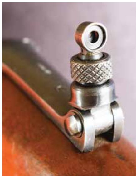
Lyman's first patented sight was a tang-mounted aperture, with a relatively big hole. Riflemen liked it!
