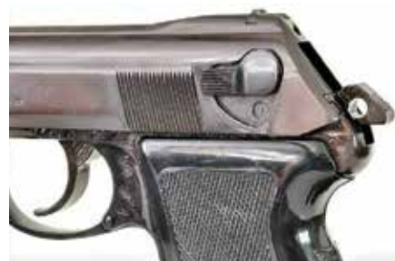
This is a standard P-64 of 1970s manufacture (above) showing the improved, triangular shaped hammer. Note the distinctive humped back and the windage adjustable rear sight. The P-64 pistol operates and field strips (below) like a Walther PPK but is different mechanically.
