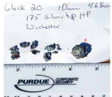
The 10mm Silvertip did massive damage to a hog it instantly killed. Core remained intact and went deep; fragments radiated outward causing corollary wound track damage.
