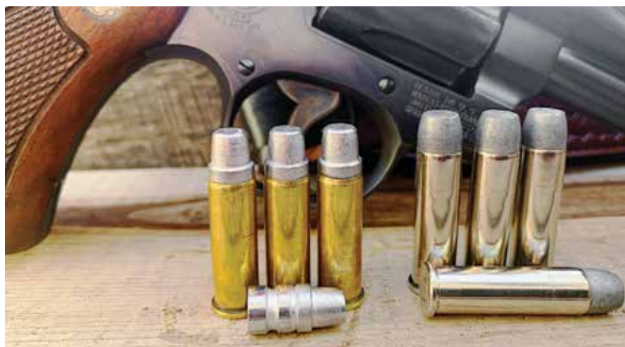
The .357 Magnum has its roots from hot loaded .38 Specials (left). Today, heavier bullets (right) like these weighing 187 grains give the .357 Magnum more punch than ever before. Evolution of the .357 Magnum (below, L to R) — Hot loaded .38 Specials, factory-swaged 158-grain .357 loads, Heavy cast .357 handloads, jacketed .357 factory loads.
