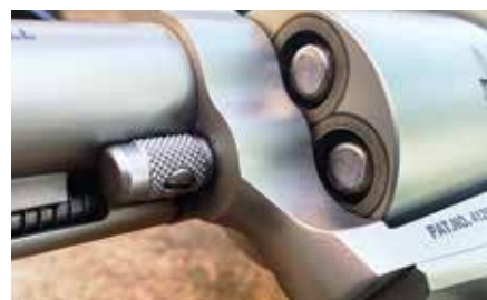
The bullet is designed to maximize powder capacity, so the crimp-groove keeps the bullet seated as far out as possible on Freedom Arms model 83s.
