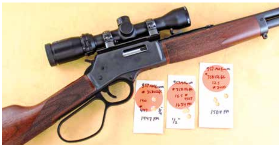
Loads with the Lyman #358156 Thompson Gas Check Bullet. John tested the .357 Magnum Henry with Black Hills 158 JHPs, 158- and 200-grain cast gas check bullets and jacketed bullets (below) from Hornady, Speer and Sierra.
