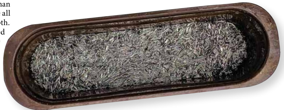
Case in collet of Power Case Trimmer (left) after being trimmed. Note the shine on the inside and outside of the case mouth as they are chamfered at the same time the case is trimmed. Lyman Cyclone Rotary Tumbler (above) takes brass cleaning to a whole new level. Media for the rotary tumbler (below) uses thousands of small stainless steel pins.
