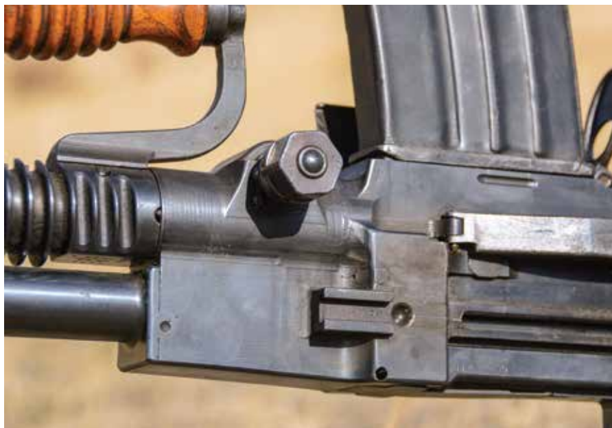
Turning this knob frees the Type 99's barrel so a cool one can replace a heated one. Wooden handle is used so barrel changer doesn't burn his hand.
