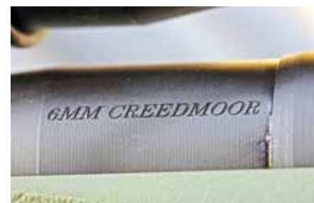
The barrel on this Ruger American Predator model in 6mm Creedmoor is made with a 1:8 twist to accommodate long, ballistically efficient bullets.
