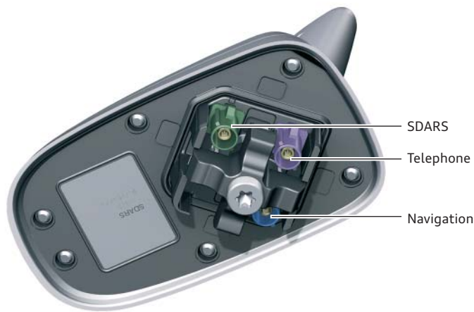
Roof aerial R216 (North America)
