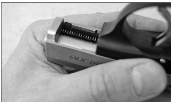
Figure 8. Recoil Spring Seated in Corner of Slide
