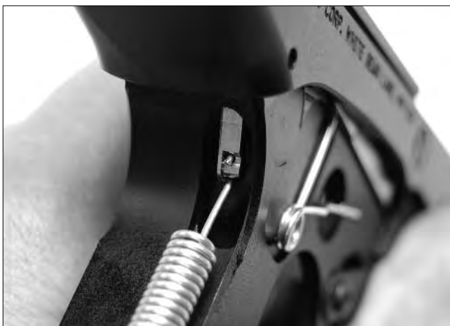
Figure 29. Correct Mainspring attachment
