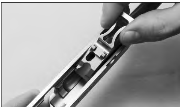
Figure 7. Installing Unlock Block
