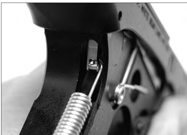
Figure 30. Incorrect mainspring attachment
