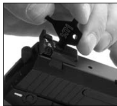
Fig. 30 Adjusting elevation screw
