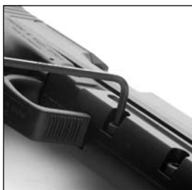
Fig. 35 Removing USP Match counterweight with 3 mm Allen wrench
