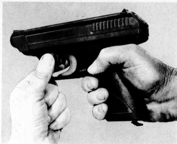
Fig. 6: Pull retaining catch downward
