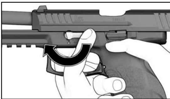
Figure 14 — Rotating the disassembly lever
