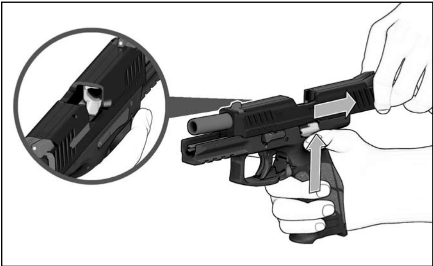
Figure 4 — Clearing the VP9 Pistol
