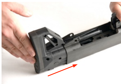
Figure E-7: Lift Firing Pin while Inserting Stock
