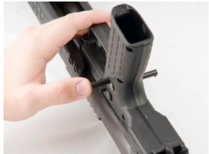
Figure D-2: Place Rear Assembly Pins in Retaining Holes
