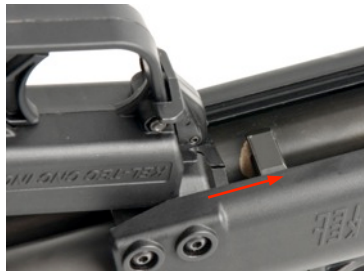
Figure E-8: Move Forend Rearward and Insert Grip Assembly
