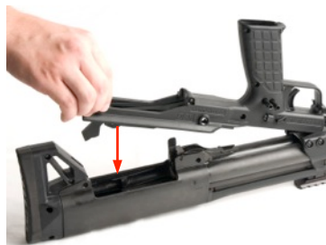
Figure E-8: Move Forend Rearward and Insert Grip Assembly
