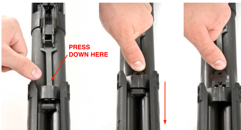
Figure D-7: Hold DFE Link Down and Slide Forend Away from Link
