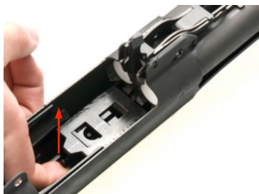
Figure E-7: Lift Firing Pin while Inserting Stock
