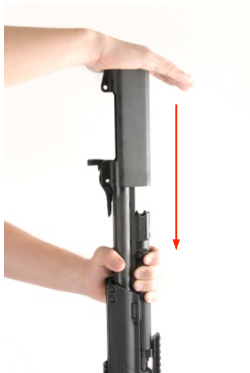
Figure E-2: Join Barrel Assembly to Receiver Assembly
