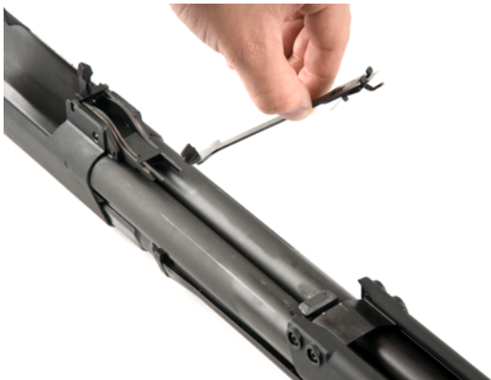
Figure D-8: Remove DFE Link before Separating Receiver & Barrel Assemblies
