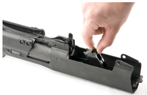
Figure D-5: Remove Exposed Bolt from Receiver
