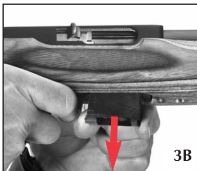
Figure 3. The safety should be “on” when the magazine is being removed or inserted. Move the magazine release forward (Figure 3A) and draw the magazine out by grasping it between your thumb and forefinger and draw it out of the magazine well (Figure 3B).
