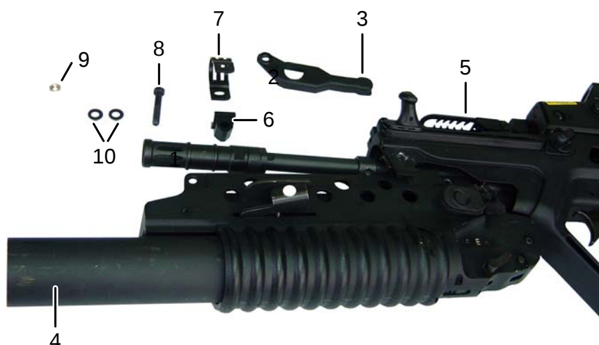
Figure 8-115. Installing the Grenade Launcher
