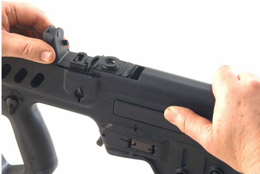
Figure 8-16. Placing Gas Cylinder into Receiver
