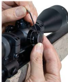
Align the windage turret cap.
